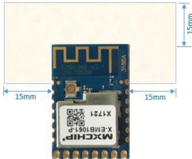
Figure 5 Minimum PCB Clearance Area
